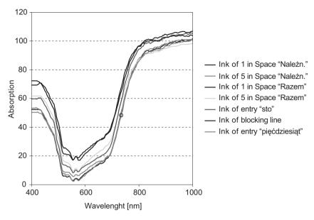
Fig. 18. Averaged reflection spectra of inks on the questioned document.
