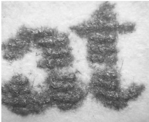
Figure 3. Lustre on the Surface of Printed letters (Thin paper)
