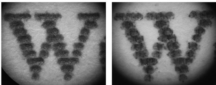
Figure 6 (a) and (b). Visibility of individual dot impression on different papers
