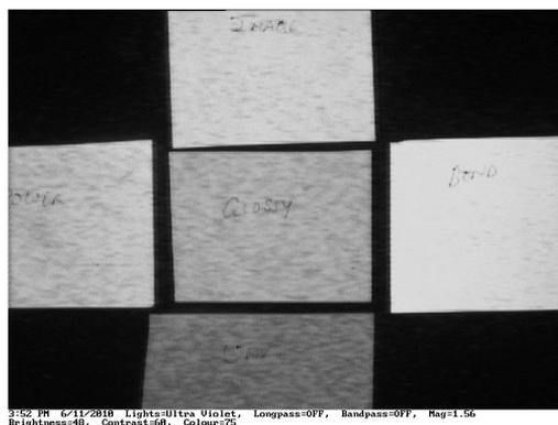
Figure 7. UV fluorescence of different paper
