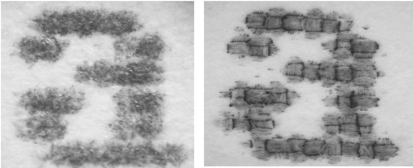
Figure 2 (a) and (b). Spreading of ink along the fibres of paper
