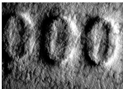
Figure 33. Letterpress — embossing effect on the rear side
