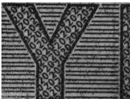
Figure 24. Intaglio: micro-text, positive printing
