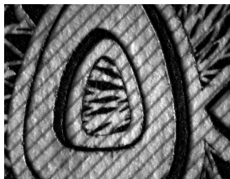
Figure 17. Intaglio: (50,000 Lebanese banknote) feathering, relief, Orlof, negative micro-text
