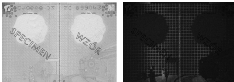
Figure 12. Anti-Stokes ink, Poland, official passport when exposed to infrared light
