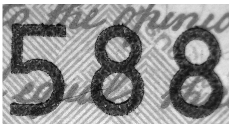
Figure 31. Letterpress — beaded edges, printing interruptions
