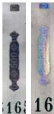
Figure 22. Optically variable effect “scate,” 500 Russian Rubles (1997), modification (2010)
