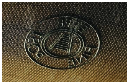
Figure 11. Electrotpe made watermark
