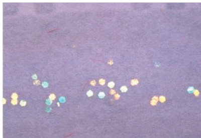
Figure 28. UV fluorescent multi-color planchettes, invisible under daylight
