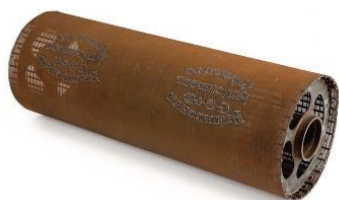
Figure 9. Dandy roll-made watermark
