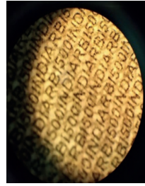
Figure 13. “RBI500INDIA” above the see-through register
