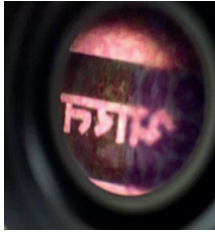
Figure 7. “Bharat” on the security wire
